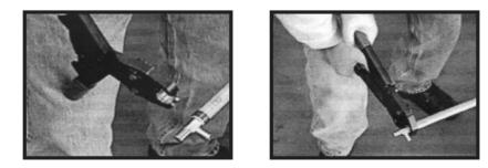
Grasp crimp ring with tool head and squeeze handles together until fully closed.
